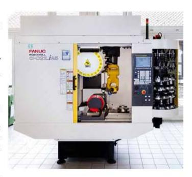
basic machine, a Robodrill a-D21LiA5, which already has a very modest footprint. The three-axis standard Robodrill was upgraded by Häberle, using proven and standardised axes, to a five-axis machine. A side panel of the machine is removed, and a carousel especially developed and built by Häberle is mounted
